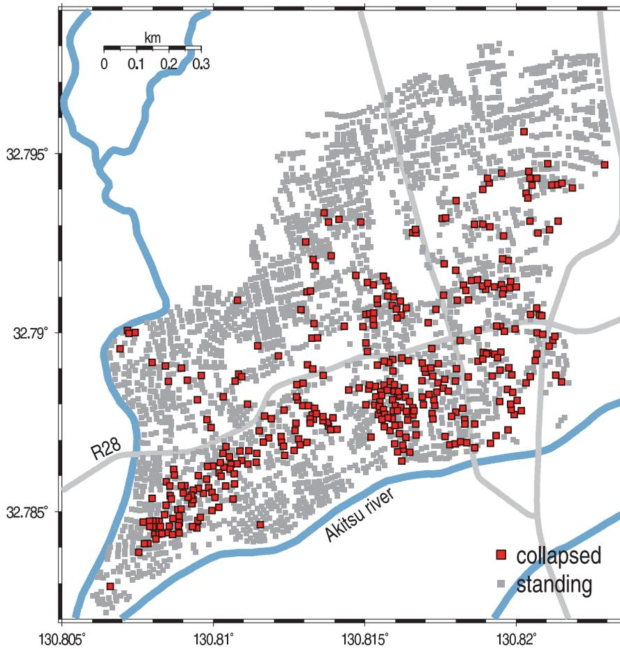
**Figure 10.** Distribution of collapsed buildings detected from the aerial photo analysis after the April 16 event.
