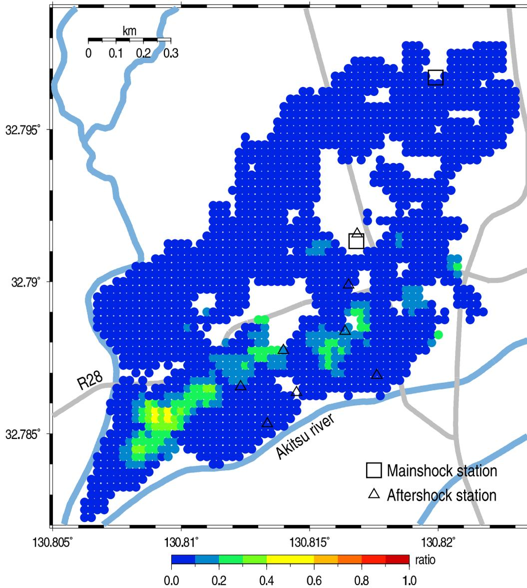
**Figure 6.** Ratio of collapsed buildings detected from the aerial photo analysis before the April 16 event. The square and triangle symbols are the same stations as those indicated in Figure 2.
