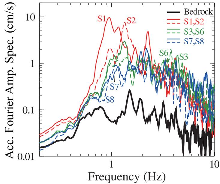
**Figure 14.** Fourier amplitude spectrum of EW component for the aftershock. Black line shows the KiK-net borehole record, and colored lines show the records at temporal stations shown in Figure 2.
