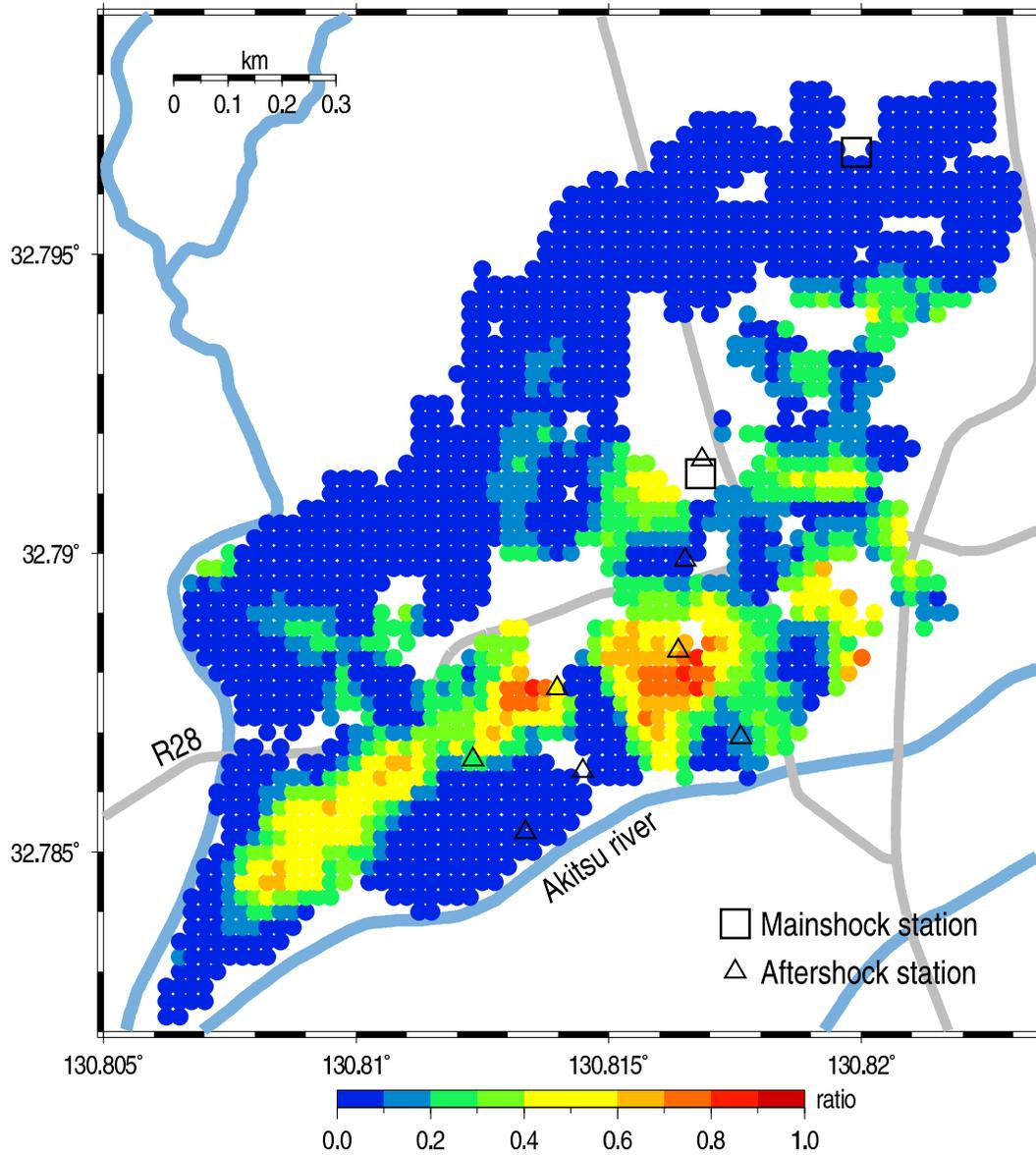
**Figure 7.** Ratio of collapsed buildings detected from the aerial photo analysis after the April 16 event. The square and triangle symbols are the same stations as those indicated in Figure 2.
