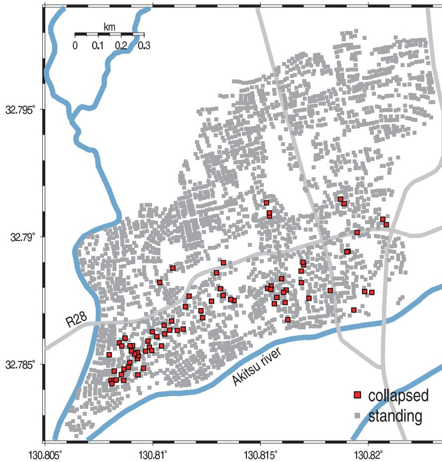
**Figure 9.** Distribution of collapsed buildings detected from the aerial photo analysis before the April 16 event.
