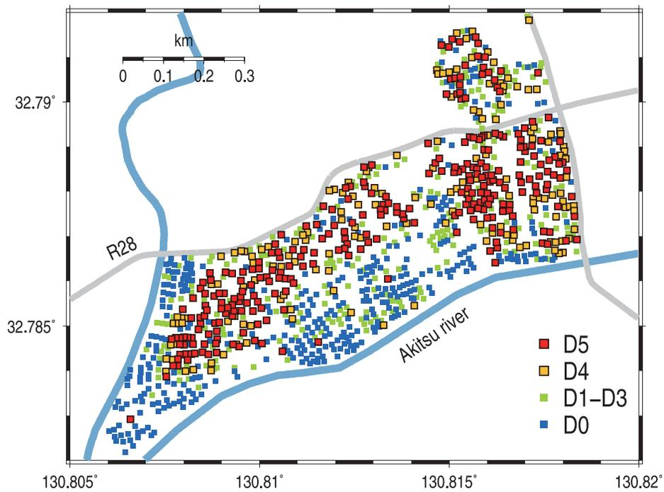
**Figure 8.** Distribution of damaged buildings detected from the field survey conducted in June 2016. Colors show the damage level.
