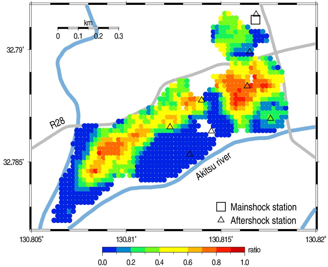
**Figure 5.** Ratio of D5 (story-collapsed) wooden buildings detected from the field survey conducted in June 2016. The square and triangle symbols are the same stations as those indicated in Figure 2.
