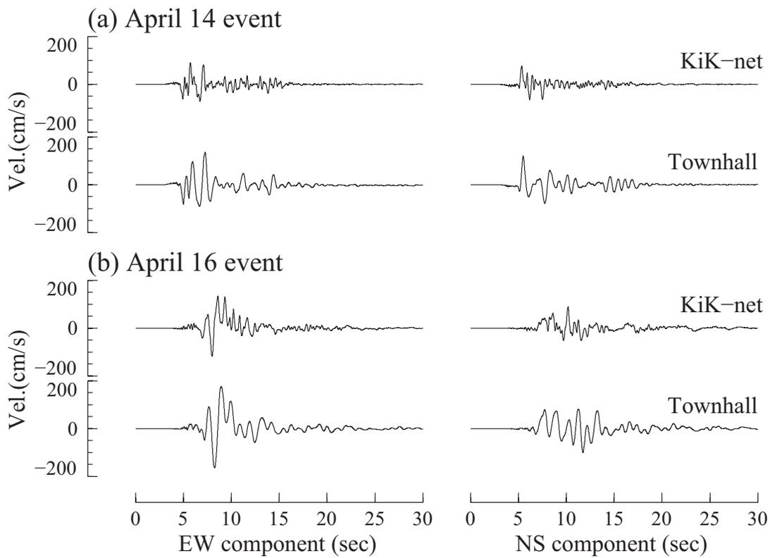
**Figure 3.** Velocity waveforms for (a) April 14 and (b) April 16 event. Locations of the stations are shown in Figure 2.
