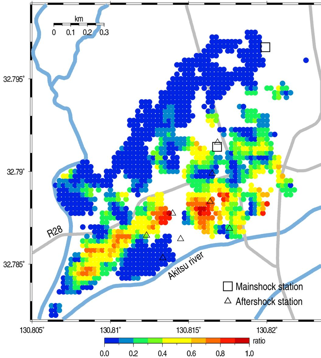
**Figure 13.** Ratio of collapsed buildings that were constructed between 1967 and 1986, detected from the aerial photo analysis after the April 16 event.
