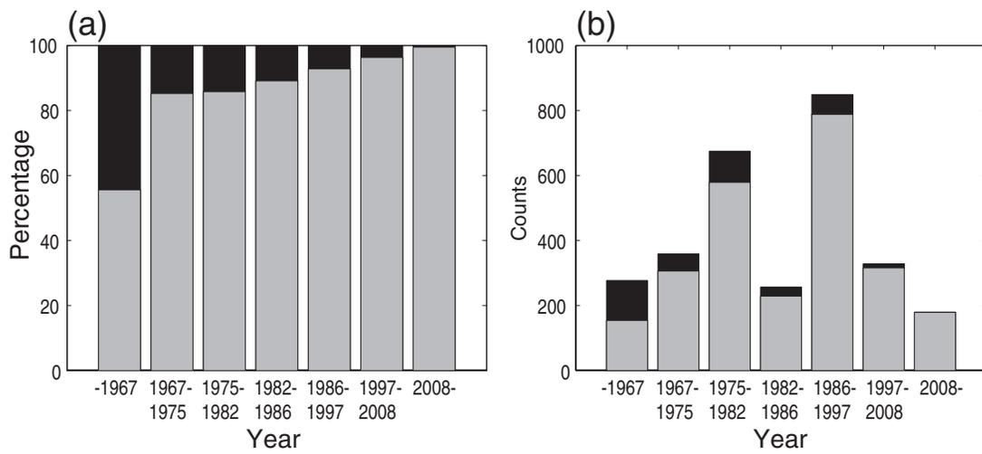
**Figure 11.** (a) Percentage and (b) number of collapsed buildings (black) and standing buildings (gray) for different building construction periods.
