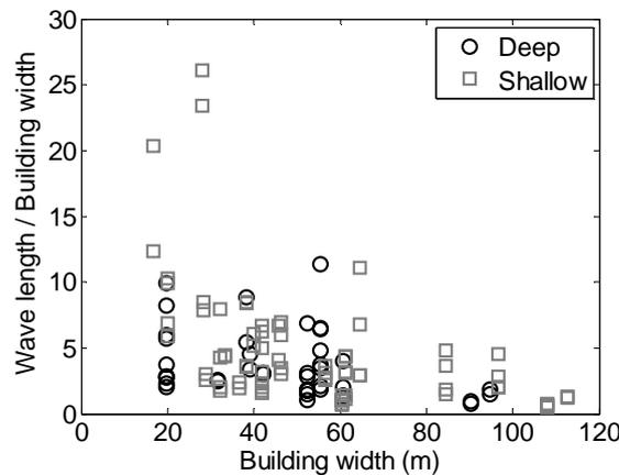
Figure 8. Relationship between the building width and the ratio between the wave length and building width.
