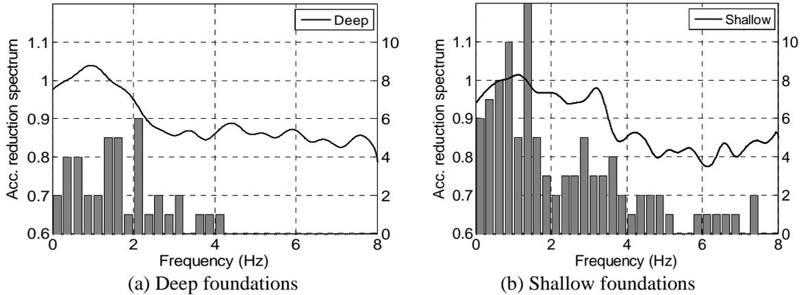
Figure 13. Acceleration reduction spectrum in Figure 11 and histogram of natural frequency of structures.
