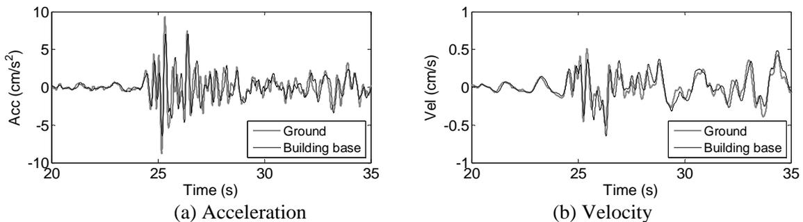
Figure 2. Comparison of the waveforms recorded at the building base (black) and associated free field (gray).
