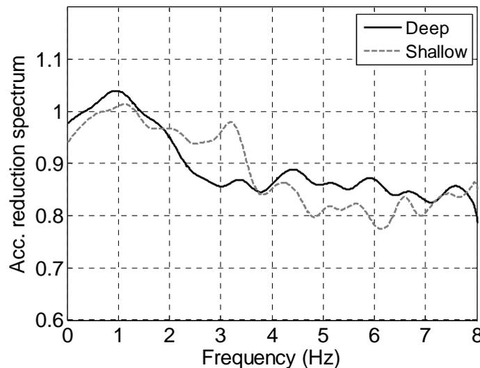
Figure 12. Average reduction spectrum for deep and shallow foundations.
