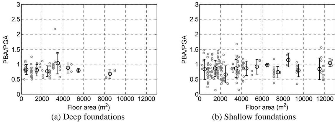
Figure 7. Relationship of the floor area and acceleration reduction ratio.
