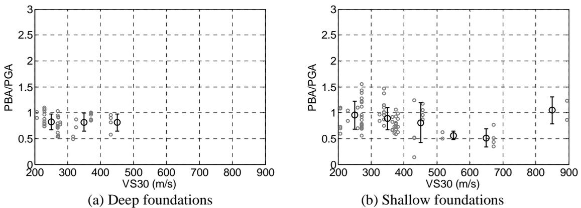
Figure 10. Relationship of the VS30 and acceleration reduction ratio.
