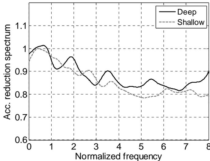
Figure 14. Average reduction spectrum for deep and shallow foundations normalized by the natural frequency of each structure.
