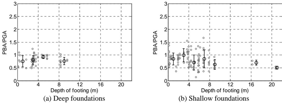
Figure 9. Relationship of the depth of footing and acceleration reduction ratio.
