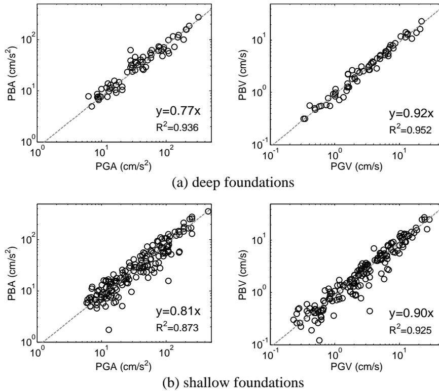
Figure 6. Relationship of the ground motion measures recorded at the free field and building base.
