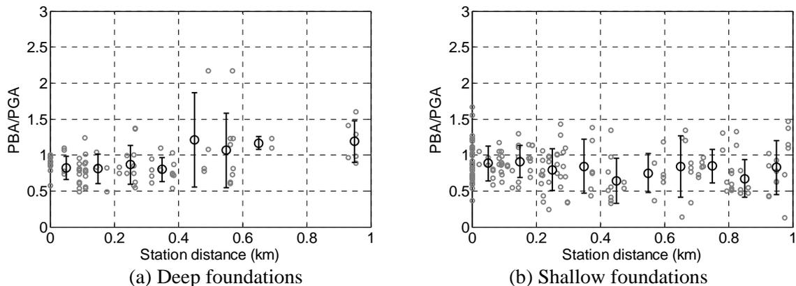
Figure 5. Relationship between the station distances and the ratio of the peak acceleration (PBA/PGA). The black circles show the median of the data with the increment of 0.1 km, and the error bar shows the standard distribution.
