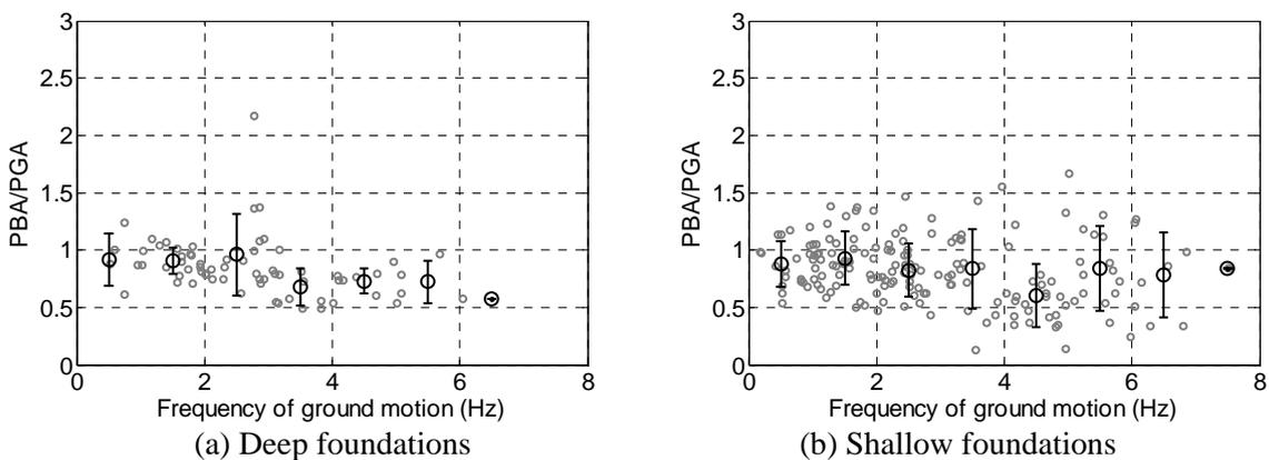
Figure 11. Relationship of the frequency of the strong motion and acceleration reduction ratio.
