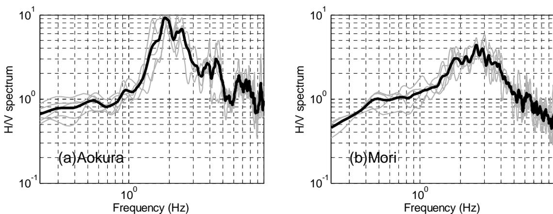
**Figure 6.** Typical H/V spectra of ambient noise in Aokura and Mori colonies. The thin lines show the spectra of 5 segments, and the thick line shows the mean spectrum of 5 segments.
