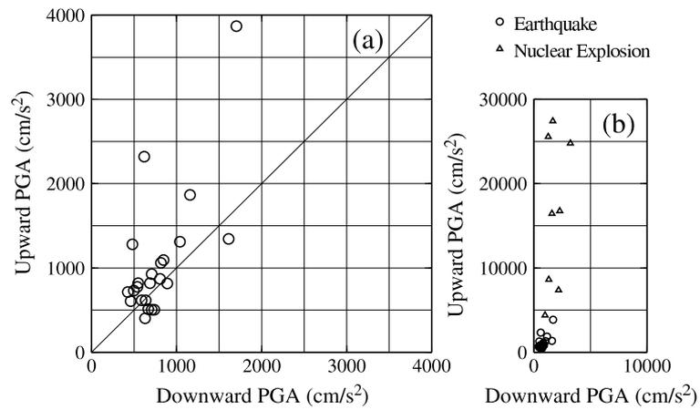
Figure 5: Relationship between the upward and downward PGA for large acceleration records.
