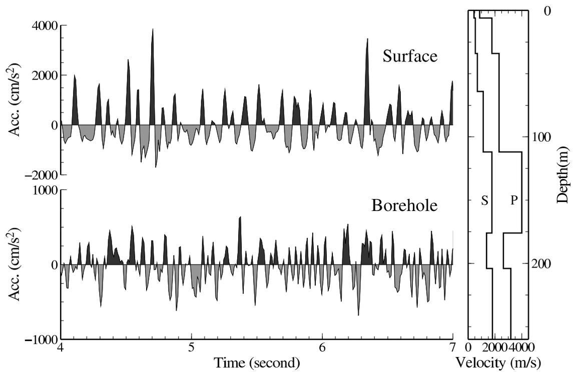
Figure 3: Expanded view of acceleration waveforms of station IWTH25. Top is the surface record and bottom is the borehole record. The right figure shows P- and S-wave velocity structures at the station.
