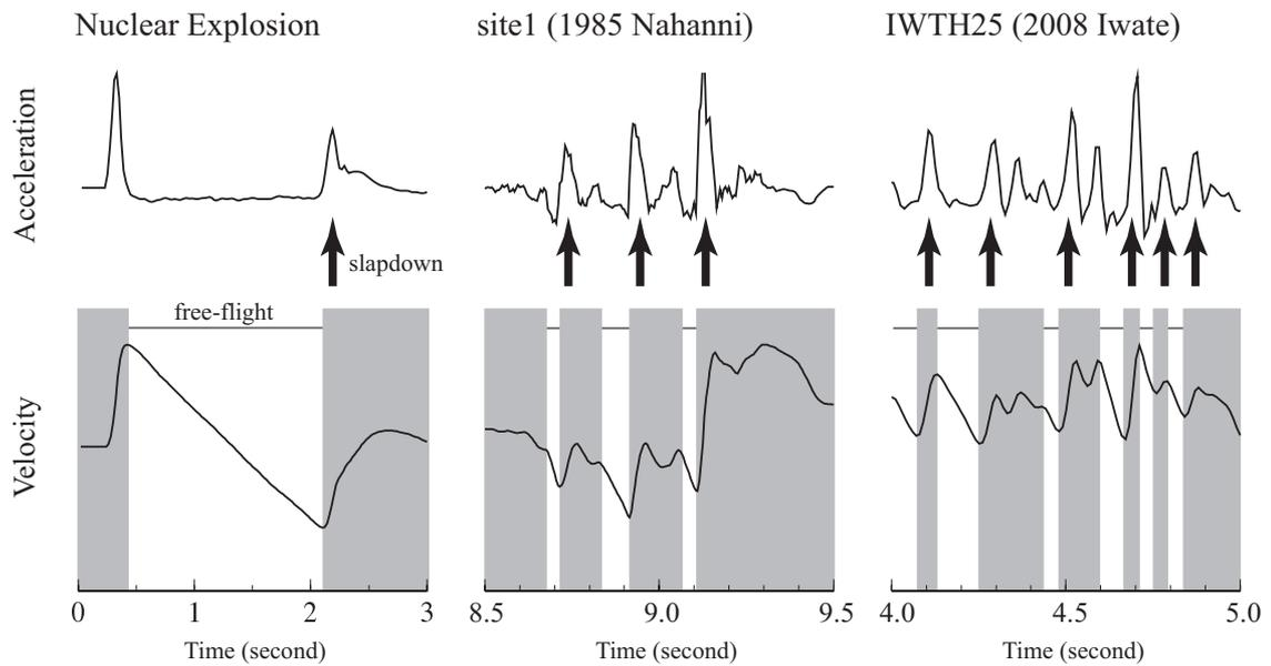
Figure 6: Slapdown phase observed in the record of the nuclear explosion on Perret (1972), site1 during the 1985 Nahanni earthquake, and IWTH25 during the 2008 Iwate-Miyagi Nairiku earthquake.
