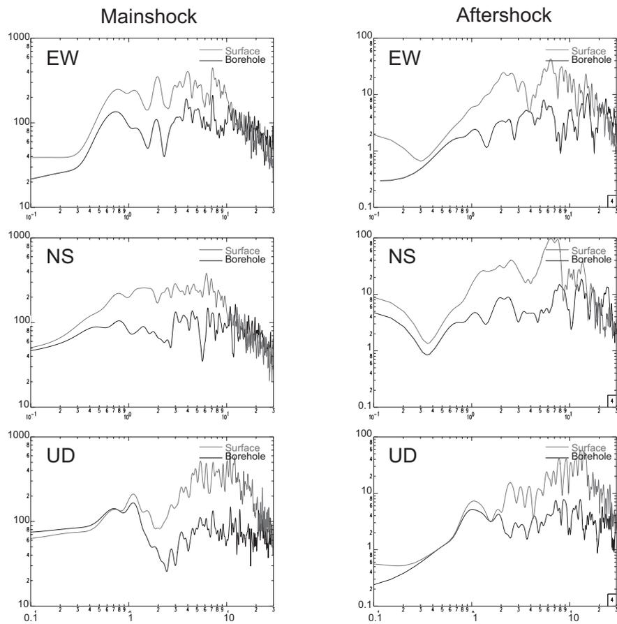
Figure 2: Acceleration amplitude spectra at the station IWTH25 in the EW, NS, and UD components from the top. The black and gray lines show the borehole and ground surface records, respectively. The left column is for the mainshock, and the right column is for the largest aftershock ( $M_j$  5.6).
