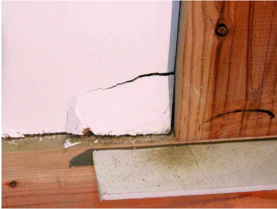
Photo 3 : [Plaster-wall test] Crack on a plaster surface.
