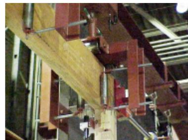
Photo 1. Appliance for supporting specimen in static tests.
