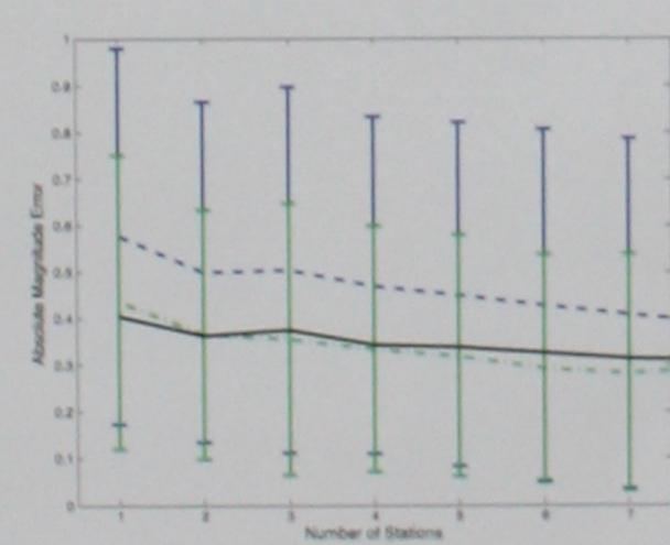
Magnitude is also dependent on the number of stations providing Pd and Tpmax data. Magnitude error decreases as additional stations trigger.
