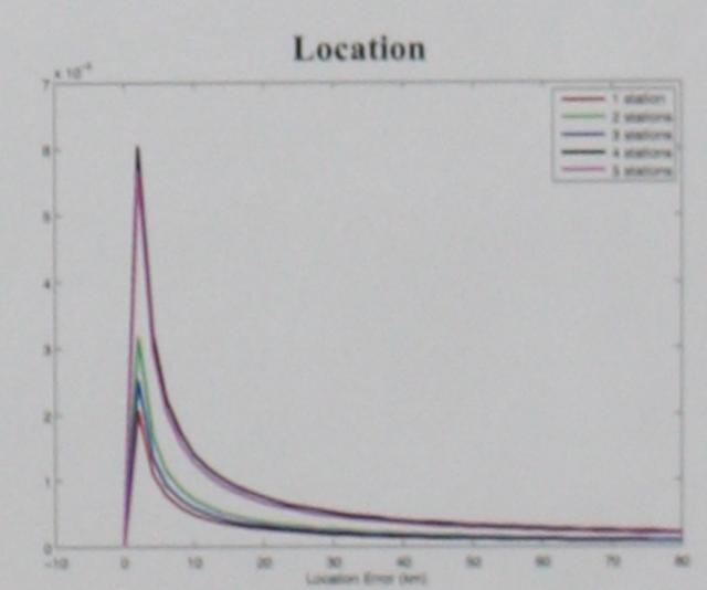
Location estimates are dependent on the number of stations providing P-wave trigger times.
