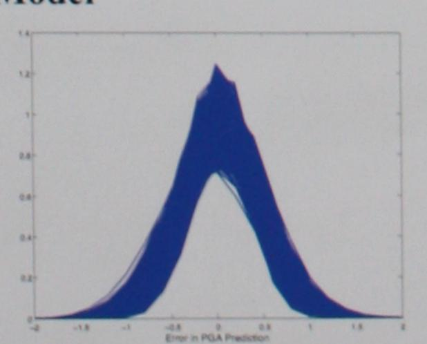
1086 error distributions created by the model. Each distribution corresponds to a unique combination of data inputs.
