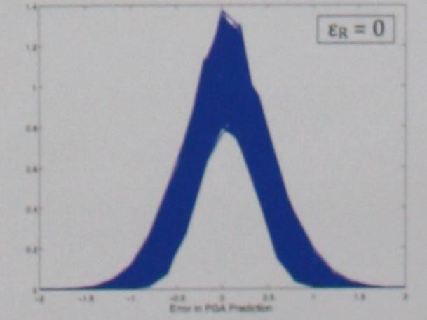
Probability distributions from error model when location error is set to zero.
