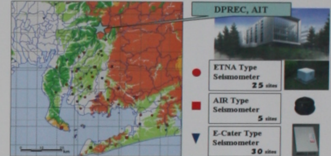
Fig.2 Network system in Mikawa Area installed by DPREC. Triangular symbols show the sites (companies) where EEW receiving terminal system and E-catcher type small seismometers are installed. Open circles and squares show the places where ETNA type seismometers and AIR type seismometers are installed respectively.
