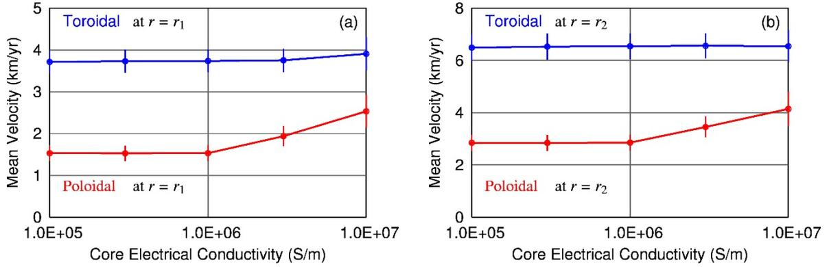
**Fig. 2.** Mean toroidal and poloidal velocity with respect to the core electrical conductivity. Circles and error bars represent means and  $\pm$  standard deviations, respectively, obtained for COV-OBS.x1 (Gillet et al. 2015) ranging from 1880 to 2015, at (a)  $r = r_1$  and (b)  $r = r_2$ .
