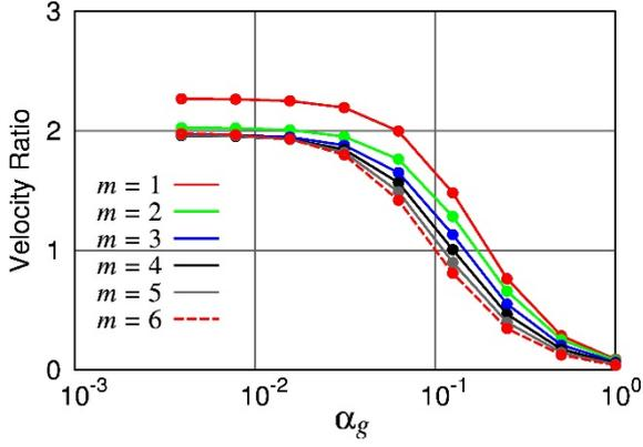
**Fig. 3.** Control parameter,  $\alpha_g$ , dependence of toroidal and poloidal mean flow ratios. Circles represent the ratio of the mean toroidal flow to the mean poloidal flow magnitudes at  $r = r_2$  under the tangentially geostrophic constraint, for spherical harmonic order  $m = 1$  to  $m = 6$ .
