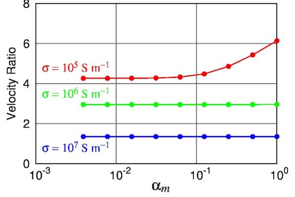
**Fig. 4.** Control parameter,  $\alpha_m$ , dependence of toroidal to poloidal mean flow ratios. Circles represent the ratio of the mean toroidal to the mean poloidal flow magnitudes at  $r = r_2$  under the tangentially magnetostrophic constraint, for  $\sigma = 10^5 \text{ S m}^{-1}$ ,  $\sigma = 10^6 \text{ S m}^{-1}$ , and  $\sigma = 10^7 \text{ S m}^{-1}$  at the epoch of 2010.
