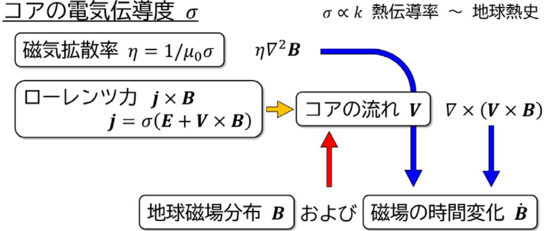
**Fig. 0.** Schematic view of relationship among effects of motional induction, magnetic diffusion, and Lorentz force on the core flow and the geomagnetic field.
