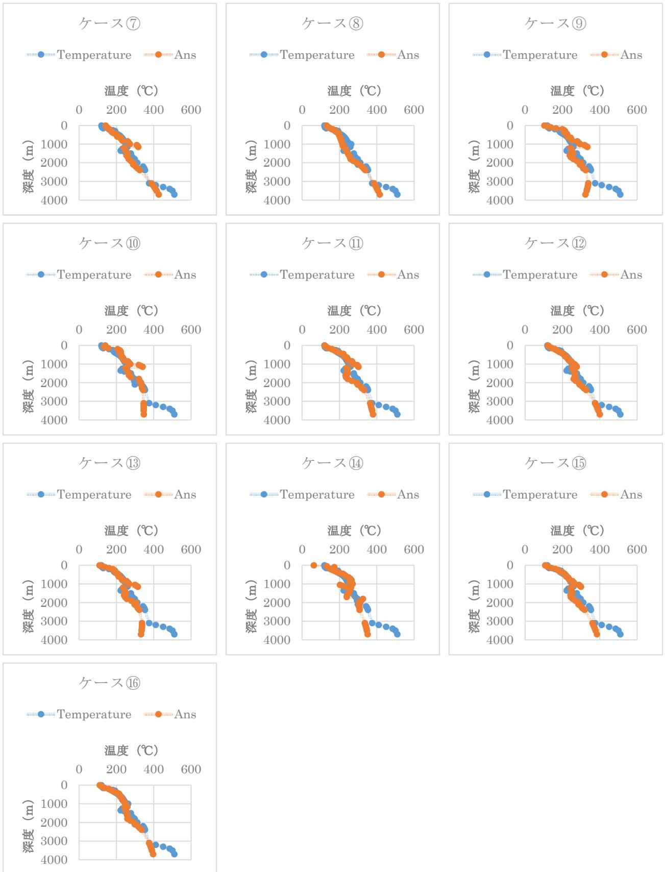
**Fig. 3** Result of temperature estimation for all cases. Blue lines indicate measured temperature, red lines indicate estimation temperature using ANN.
