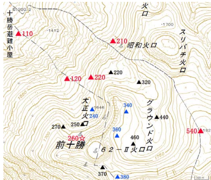
Fig.4 Sites of AMT survey on Tokachidake volcano. Blue, Black and Red triangles indicate survey points in 2009, 2014 and 2015, respectively. Star indicates a point that surveyed every time. Topographic map is GSI maps.
