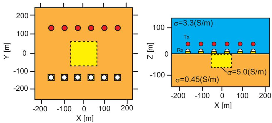
Figure 1: The synthetic model with a 3D alignment of transmitter and receivers consisting of conductive anomaly, seawater and resistive basement.
