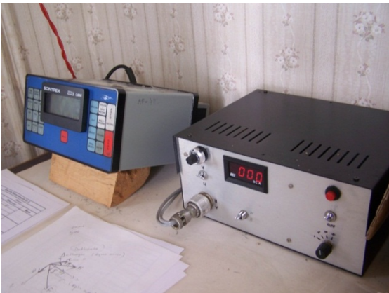
Figure 5. (a) ISK Absolute Measurement Instruments (b) Scintrex EDA OMNI Portable Proton Magnetometer
