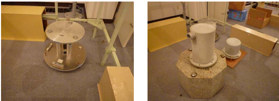
Fig. 3 Fluxgate sensor mounting stands for setting the calibration coil. Left: aluminum stand, Right: vinyl chloride stand.
