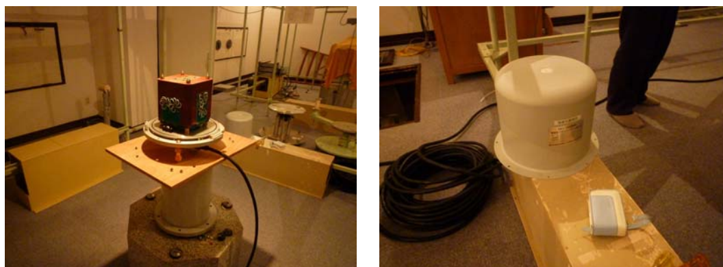
Fig.5 Uncovered fluxgate magnetometer sensor (left), and removed cover (right).
