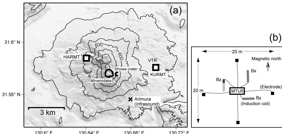
**Fig. 1.** (a) Topographic map showing the locations of MT sites at Sakurajima volcano (squares). (b) Layout of the MT measurement system. A Phoenix MTU5 system was used to measure variations in the electric ( $E_x$  and  $E_y$ ) and geomagnetic field ( $B_x$ ,  $B_y$ , and  $B_z$ ), where magnetic north (x), magnetic east (y), and downward (z) are assigned positive values.
