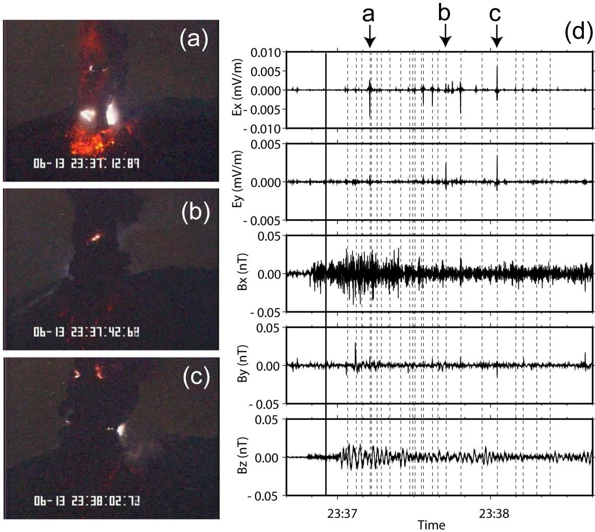
**Fig. 2.** Photographs of an eruption at Showa crater at 23:37 on 13 June 2008, and corresponding magnetotelluric (MT) time series recorded at HARMAT. The solid vertical line indicates the time when the erupted material emerged at the crater rim. Dashed vertical lines indicate times when lightning flashes were observed in the movie.
